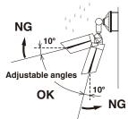
• Keep the detection window straight and the adjusting part at the bottom.
