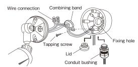
(4) Fix the mounting base tightly to the mounting box by the 2 screws.
