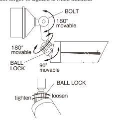
\* Keep the detection area downwards to avoid sun ray influence and other unexpected detectable objects remotely located when installing outdoors.
